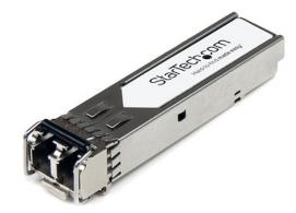
The 0231A0A6-ST is a HP 0231A0A6 compatible fiber transceiver module that has been designed, programmed and tested to work with HP brand switches and routers. It delivers dependable 10 GbE connectivity over fiber cable, for 10GBase-SR compliant networks, with a maximum distance of up to 300 m (984 ft).
